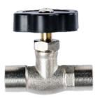
The needle valve is named for the conical stem that acts as a plug over a small diameter orifice. It can function as a restriction fitting, but with the possibility of regulating the choke in the passage section.
