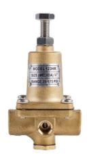
The model 123HR pilot has the 2-way pressure reduction function acting by the diaphragm, which is in the open position given the spring pressure that acts on the diaphragm. When the pressure downstream of the valve exceeds the regulated point, the water flow is closed, thus achieving pressure regulation.
